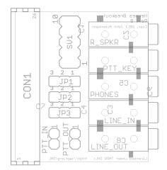
The 10-pin header (SV1) carries the 7 open-collector output signals on pins 1 though 7. The "open collector reference/flyback diodes" signal is on pin 8. Pins 9 and 10 (which are oriented nearest to the board edge) are ground.
